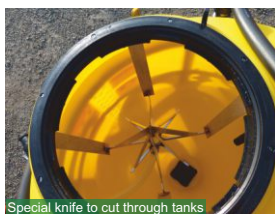
Special knife to cut through tanks
